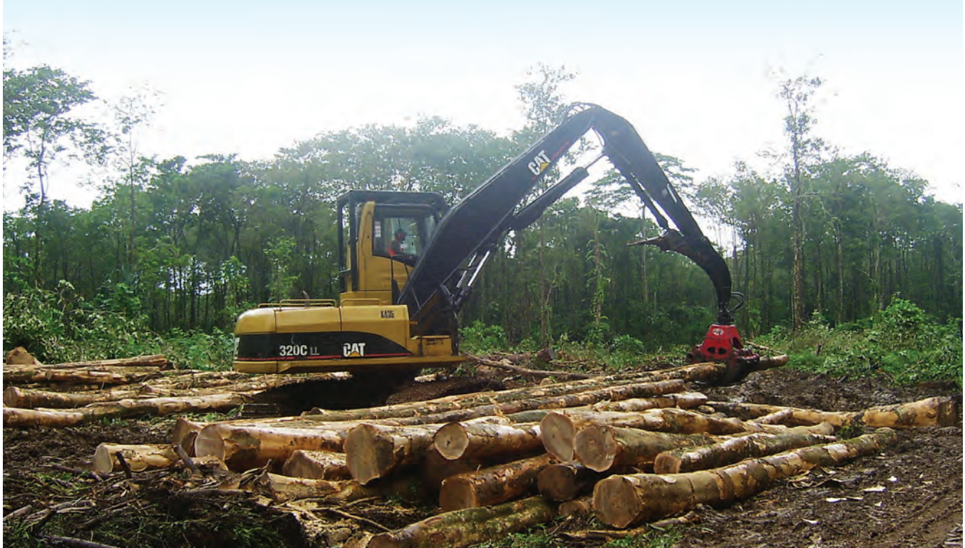
An excavator bunches logs and prepares them for loading onto a truck at Kolombangara Forest Products Limited
