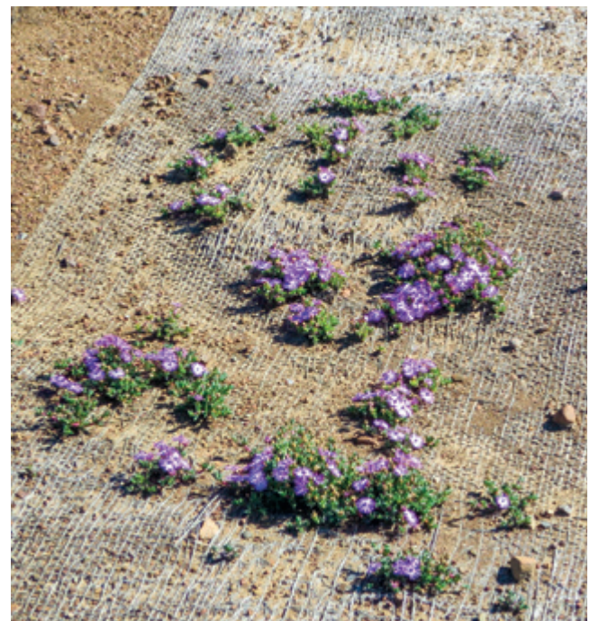
Succulent seedlings establish on previously bare surfaces covered with geotextile
