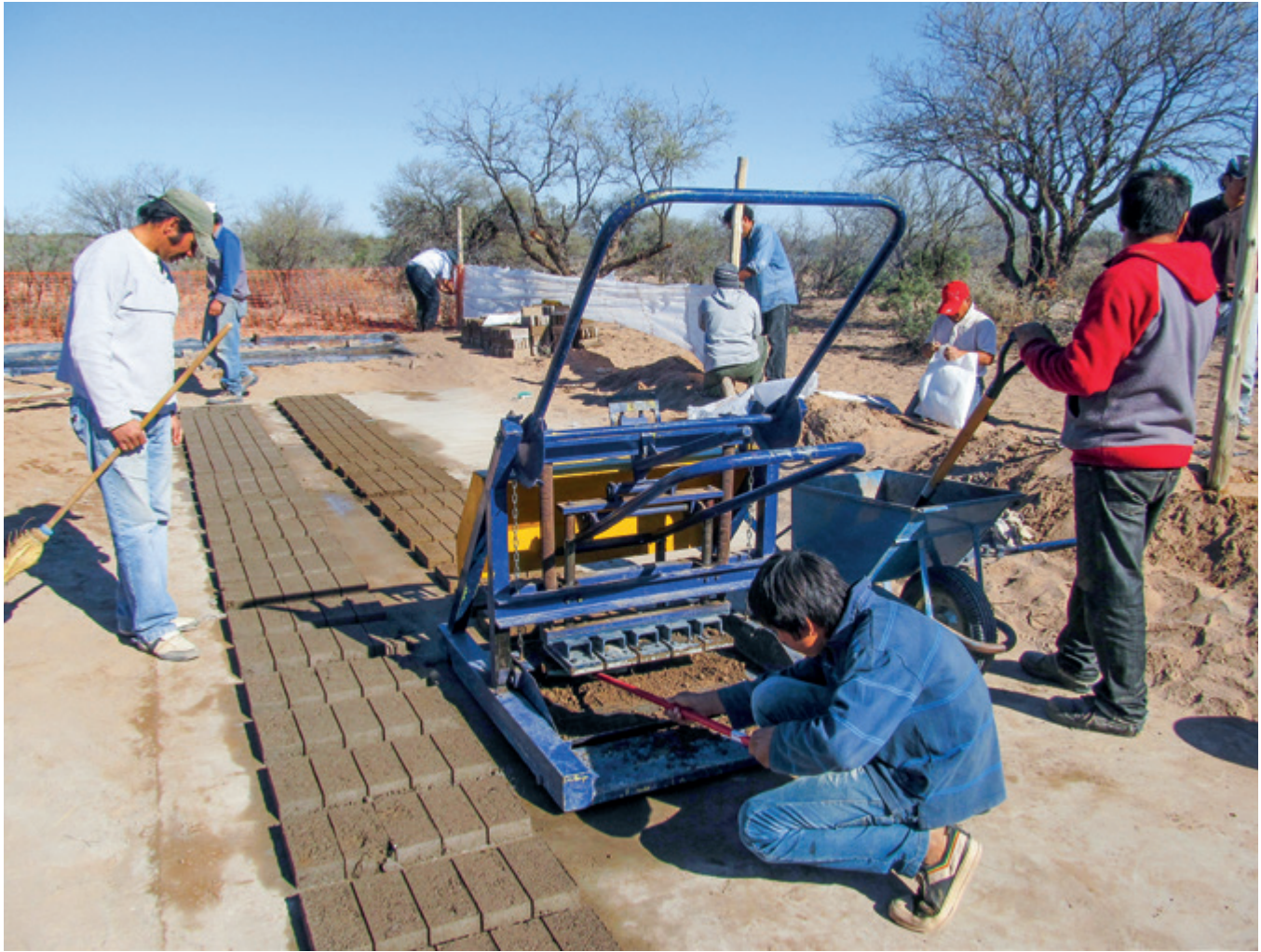
The community manufactures 'green' (unfired) bricks with local materials for the construction of the DPU
