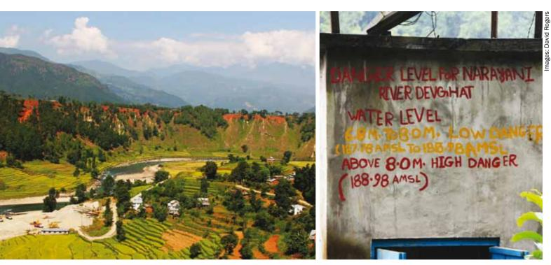
Left: typical image of Nepal, showing a river, terraces and erosion. In heavy rains landslides are common, in addition to river flooding. Right: shows flood levels on the side of a hydrological gauging station. These stations are permanently manned by an observer who takes care of the measurements and issues local alerts based on the river level and the instructions on the side of the building
