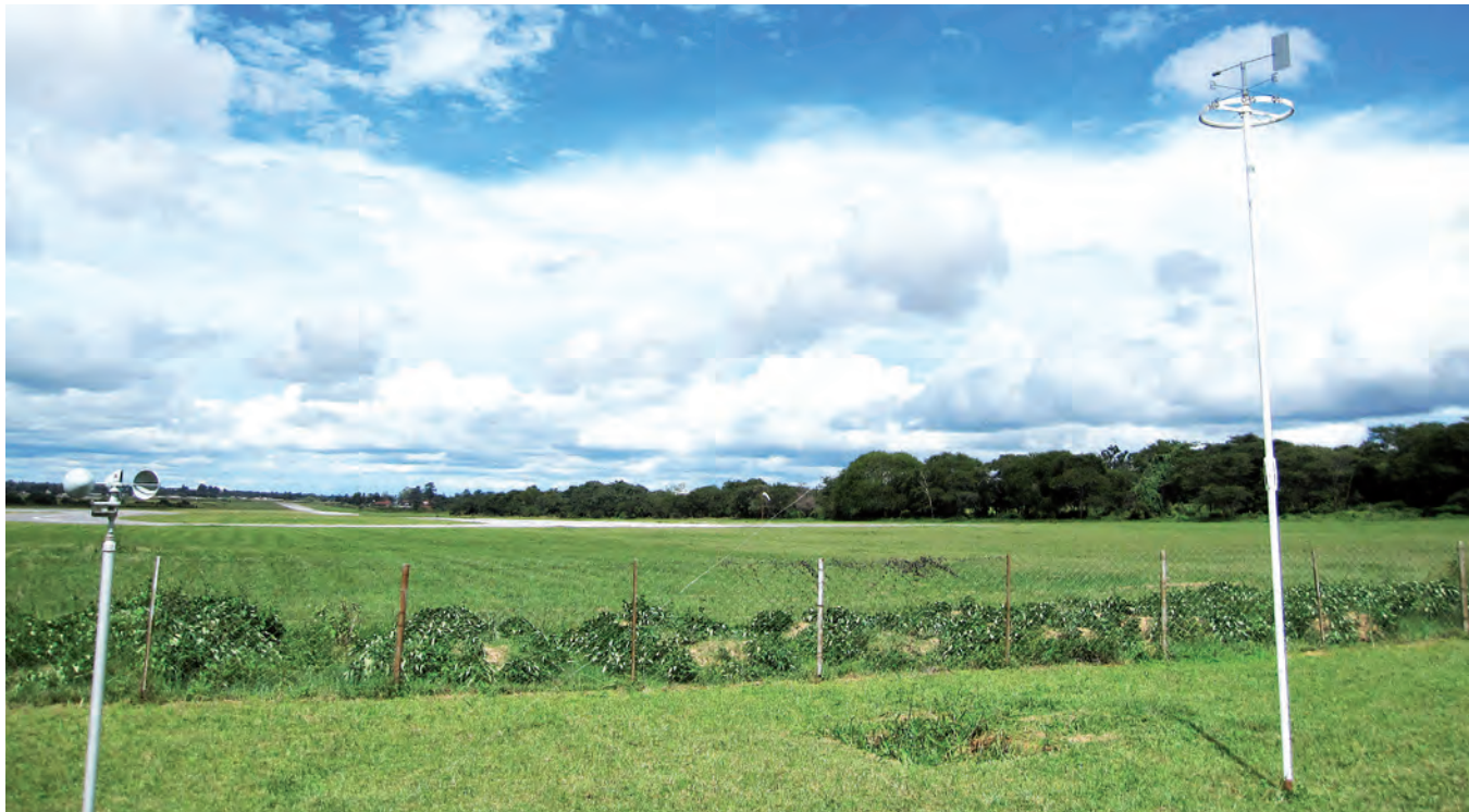
Cup counter and wind vane at meteorological station, Zambia Meteorological Department, Lusaka, Zambia
