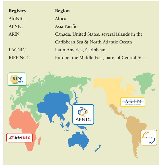
Figure 2: Address resources are managed by the five RIRs, under policies developed by their respective regional communities
