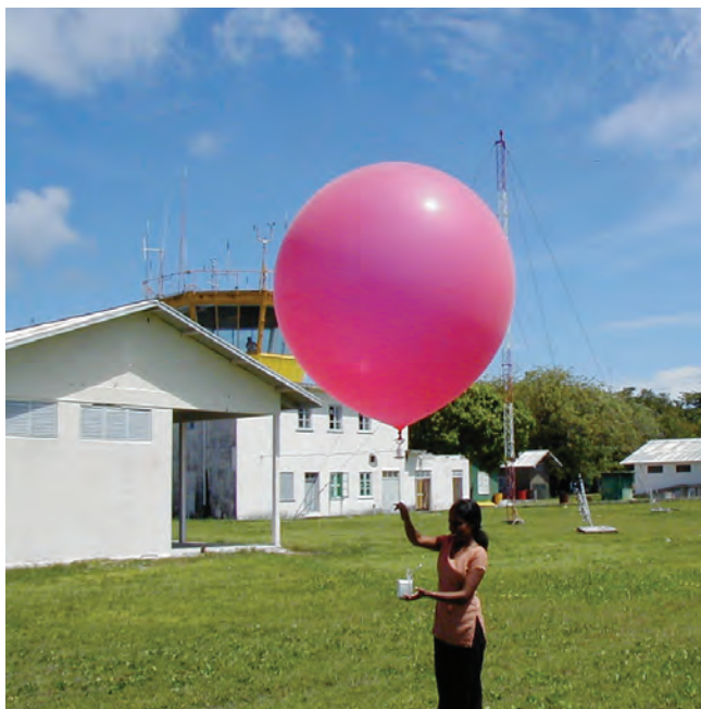
Launching a radio-sonde at Gan, Maldives after the station was re-equipped by USA and UK VCP contributions
