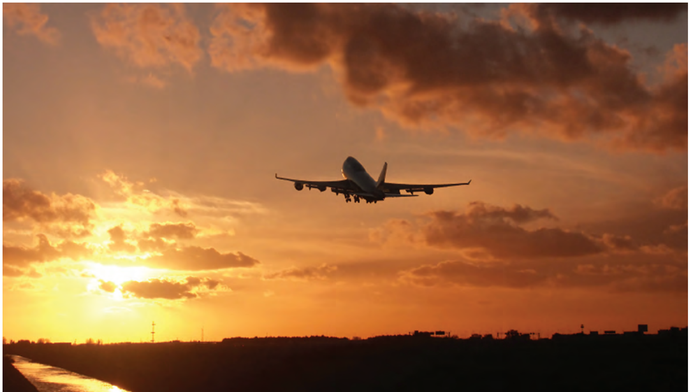
A higher temperature results in a longer take-off run because temperature affects air density
