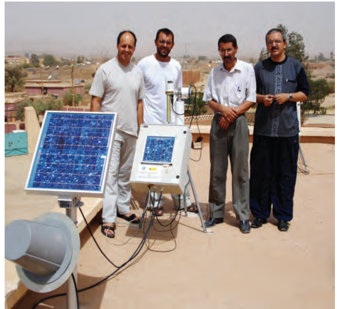
Commissioning a solar photometer at Tamanrasset in Southern Algeria with support from Spain to monitor aerosols and dust in air masses over the Sahara desert, especially for early warning of dust clouds
