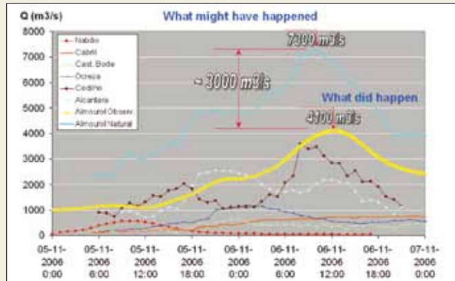
Figure 2: Peak flood attenuation of 3000 m 3 /s occurred in November 2006 in the Tagus river basin due to the cooperation between upstream (Spain) and downstream (Portugal) countries
